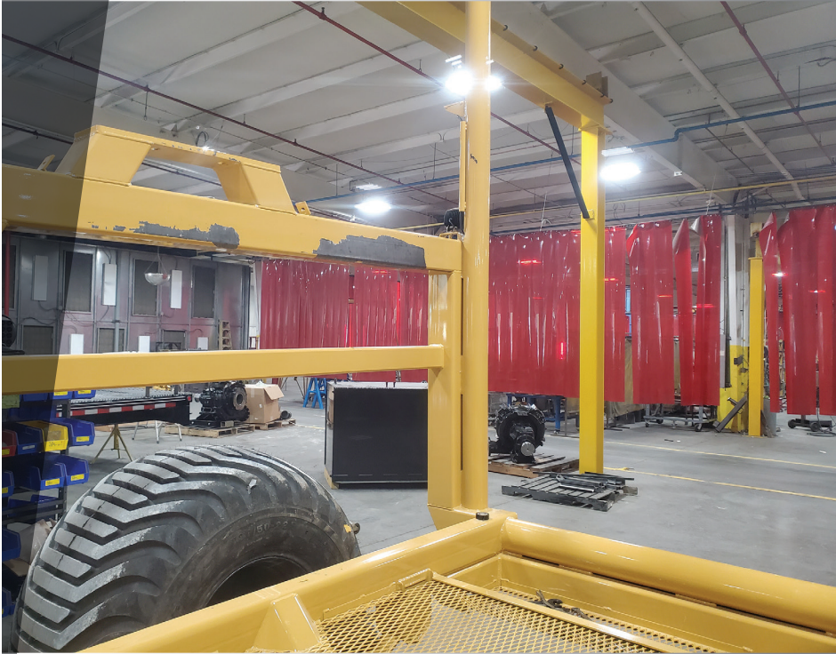
Sections of the topcoat and primer were peeling off, exposing the steel substrate.
